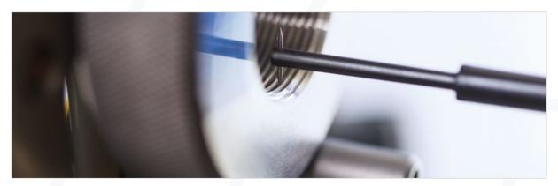
in the thread root and the roughness of the thread flanks, is only possible by modern, scanning data acquisition. Parameters that cannot be measured by "gauging" can be determined quickly and reliably, recorded, and monitored in compliance with tolerances. Optical measurement is only possible to a limited extent due to the overlap caused by the thread pitch.
