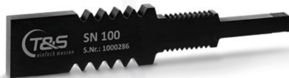
Thread standard for pitch and flank angle SN100
