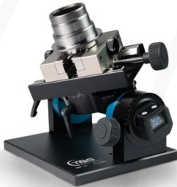
ZSR-60 with digital angle display – Jaw width 98 mm
